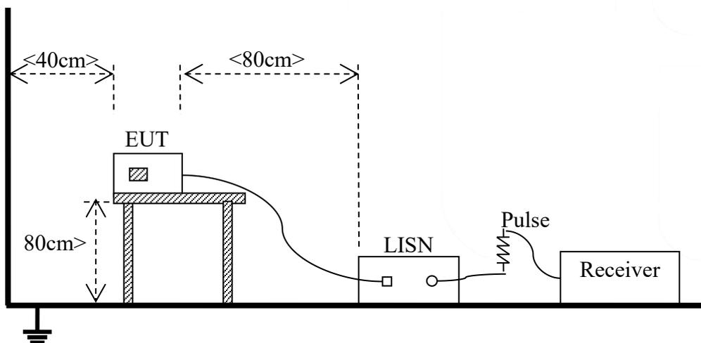
Test Setup 3 For Harmonic Current Emissions Measurement Test
