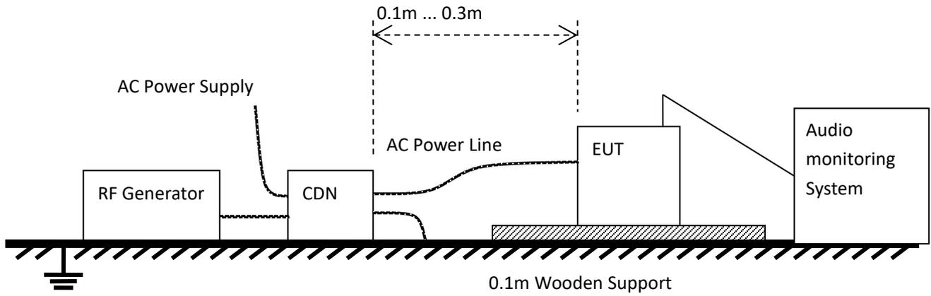
Test Setup 10 Power Frequency Magnetic Fields
