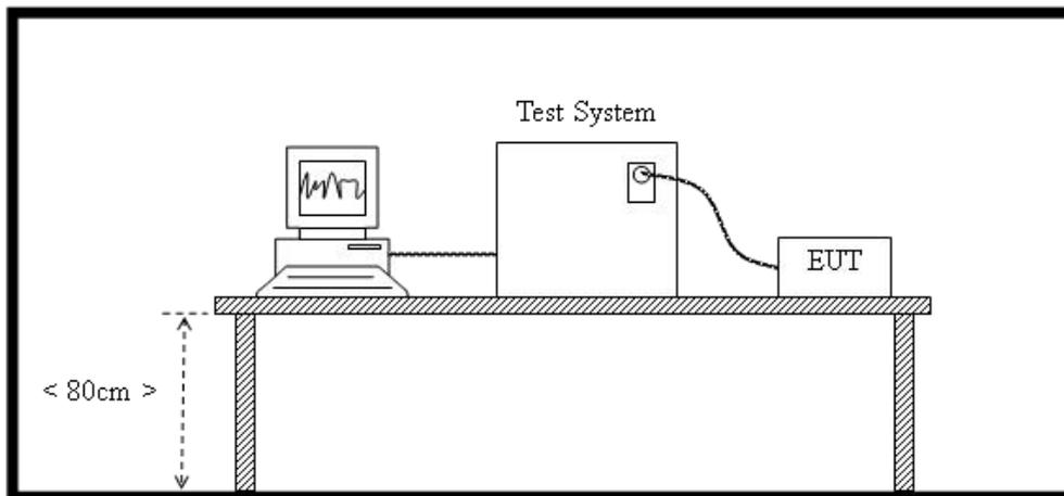
Test Setup 4 For Voltage Fluctuations and Flicker Measurement Test
