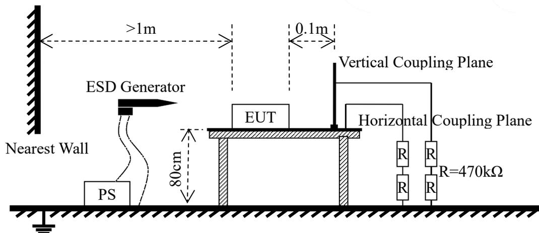
Test Setup 6 For Radiated Immunity Test
