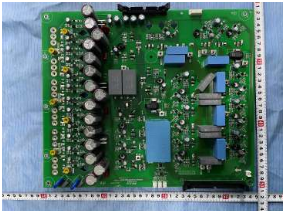
Component side of drive board for all models
