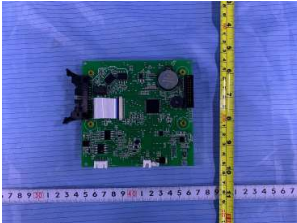
Solder side of LCD board for all models
